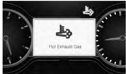
Display that notifies the operator of automatic SCR cleaning
